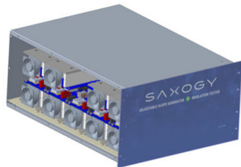
Figure 5: SAXOGY's sketch of the power unit of the dv/dt pulse generator
